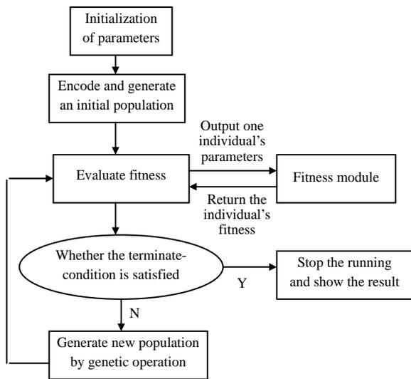
Fig.2 The framework of the genetic algorithm module
